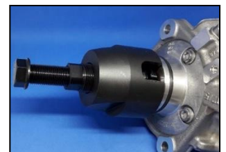
AE0301-CP4 PULLER FOR JOINT WITH 2 TEETH
