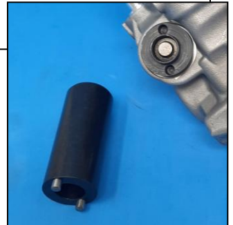
AC0539-CP4 WRENCH TO DISASSEMBLE VALVE ON PUMP CP4 similar: 0.445.011.542
