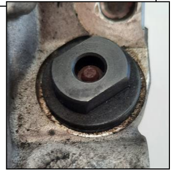
AC0530-CP4 WRENCH TO DISASSEMBLE VALVE ON PUMP CP4
